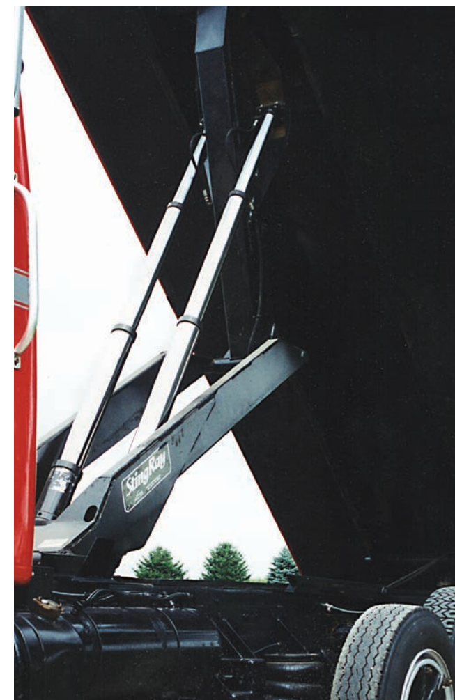
StingRay hoists are available in 5 NTEA performance classes as 1, 2 or 3 stage cylinders.
