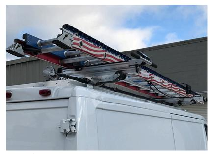
The new, simpler design makes it easier to install and adjust. The aluminum build of the rack reduces corrosion and keeps your ladder rack looking like new. It will accomodate a variety of ladders and safely secure them for transport.
